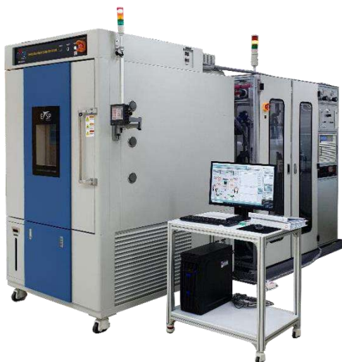
< 5kW Test Station With Temperature Chamber >
